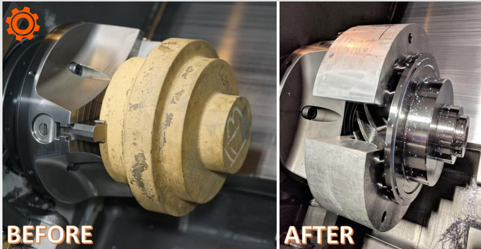
Ø18" Compressor Impeller (Material: Titanium)
