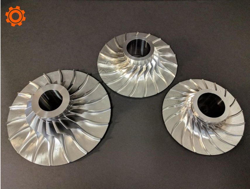
Air Compressor Impellers (Stages 1, 2, & 3) (Material: Stainless Steel)
