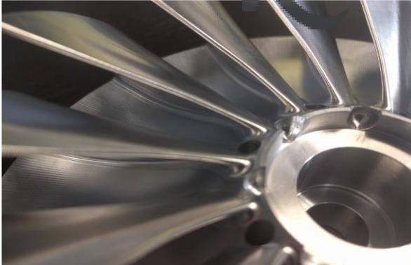
5-axis machining of turbomachinery impellers and blisks up to \text{\O}14''
