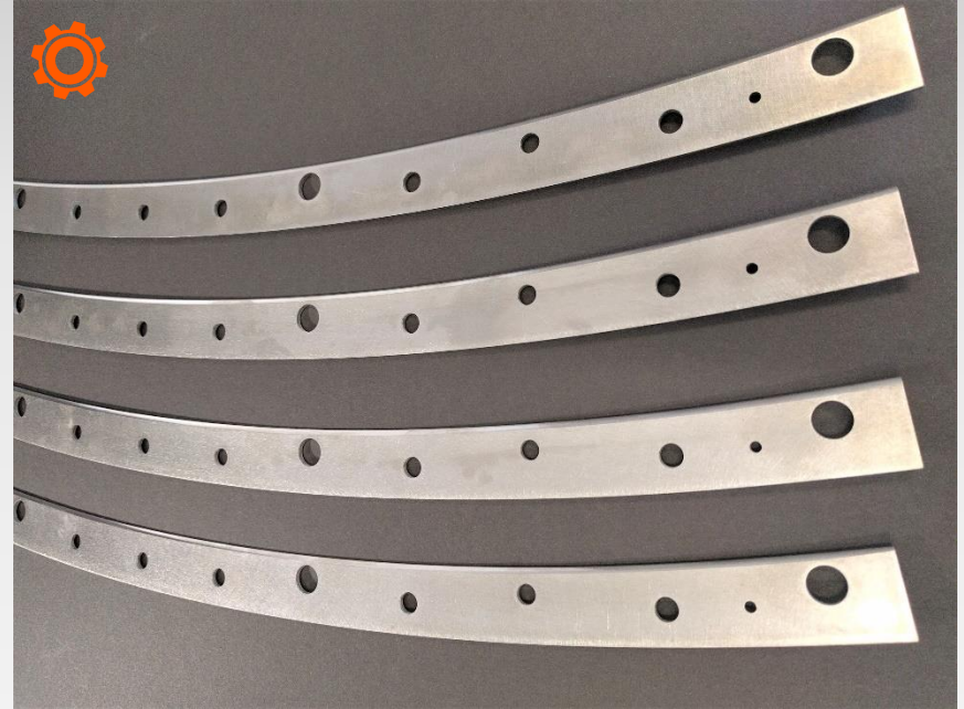
Counter-Plates for Aero-Engine Fan Case (Material: Stainless Steel)
